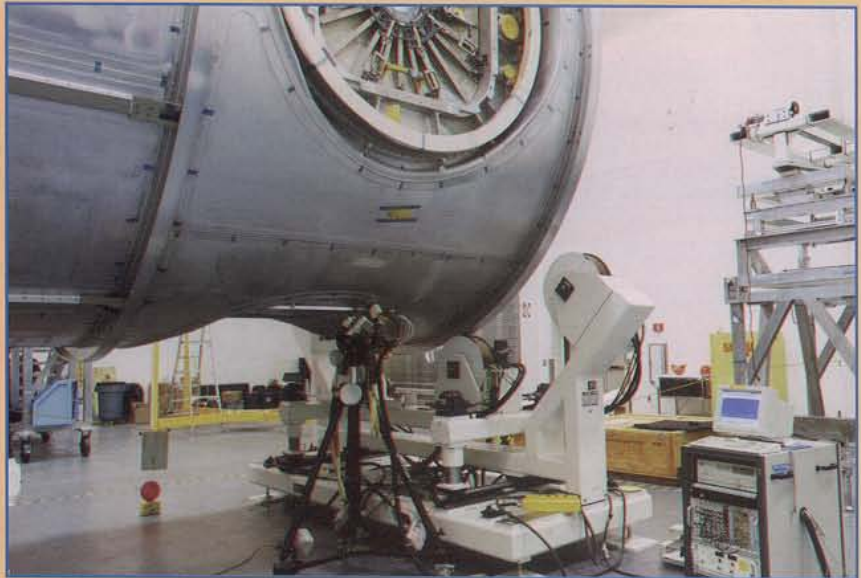
Measuring stresses on welds on the International Space Station
