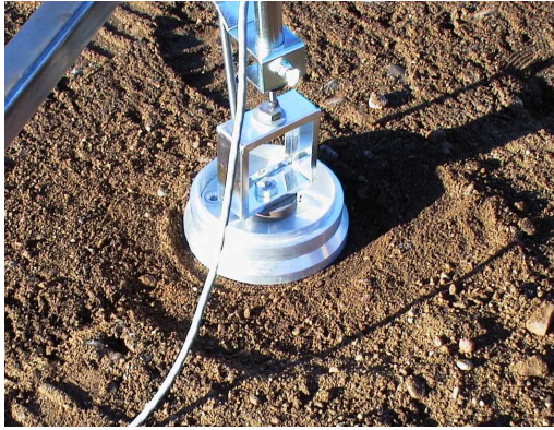
Photo 4. 4.5" Ring and LVDT
