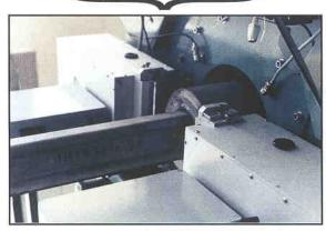
The shadow technic with parallel scanned laser beams has the advantage of measuring the object with high accuracy independent of its position in the measuring field; but only the "outer" contours like height, breadth a.s.o. can be determined by this method.
