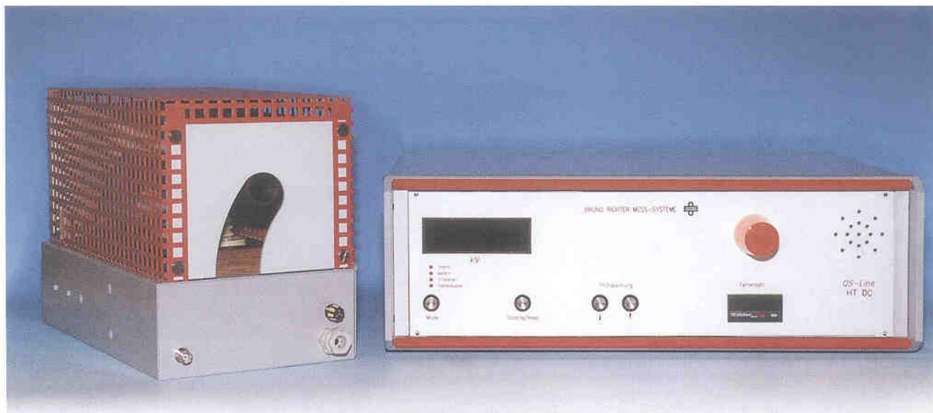
The QS-Line High Frequency Spark Tester HT-DC checks the insulation of threads and cables for pinholes and blank spots. The „HT-DC“ is especially applied when „HT-4 Sine“ cannot be used, for example in case of very thin wires, cables with thin-walled insulation or in case of very large cables with high capacitive current consumption.
